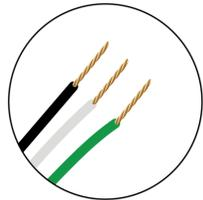
6. Connect matching wires with wire connectors and wrap secure with electrical tape.
