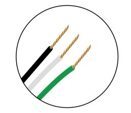
6. Connect matching wires with wire connectors and wrap secure with electrical tape.
