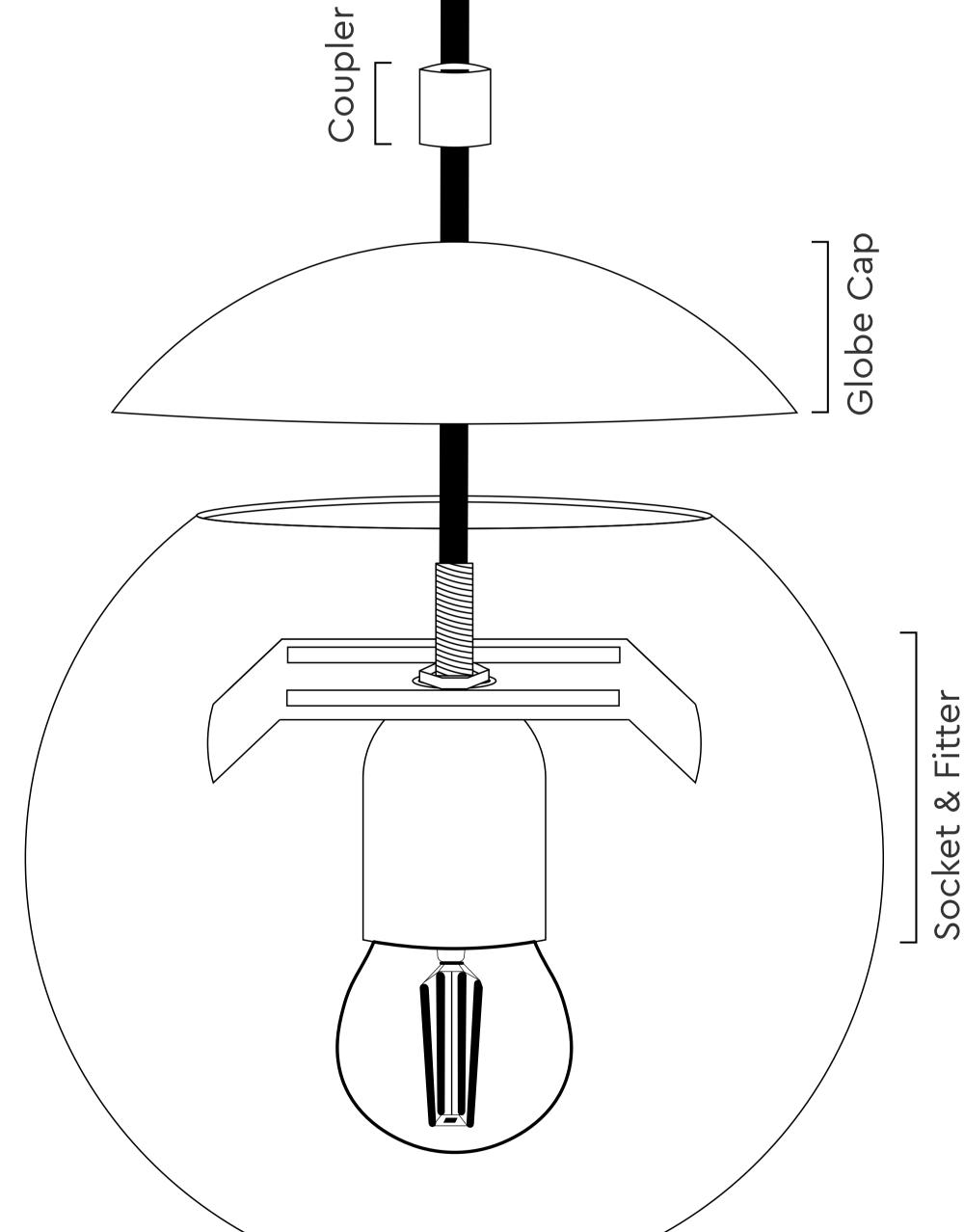
**3.** While holding glass firmly, carefully lower the fitter and socket into the globe.
